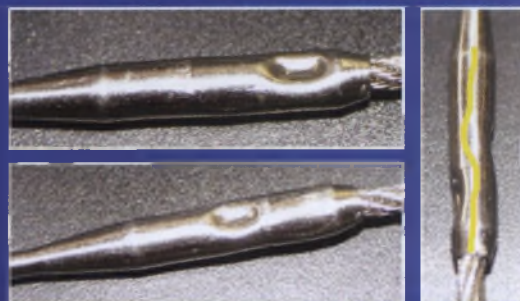
The new Paratec method; first a dimple is forged on one side (top pic), then a second offset dimple on the other (bottom pic) so the cable runs in an S-curve, this path is shown to right.
