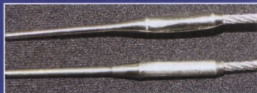
Paratec pins; the top pin, which is a flat crimp is fine, the bottom pin, which is round swaged, is suspect and needs to be tested
