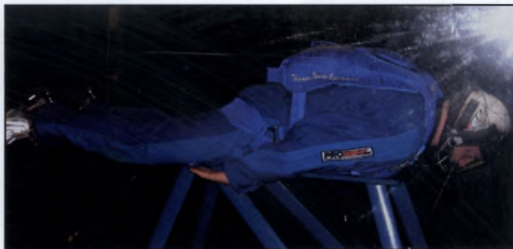
Modifying the leg of the suit to the shape below reduced drag by 20%
