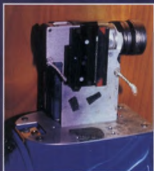
Sony PC10 top-mounted on a Headhunter Voodoo helmet. Note the supporting bracket, with bungee cord, which also acts as a bracket for a portrait stills camera or flashgun.
