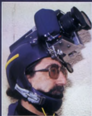
Full face system with a Sony PC9 and Nikon F90X front-mounted. (I personally wouldn't have all the weight at the front but as Tony has 4,000 camera jumps I'll let him off!)
